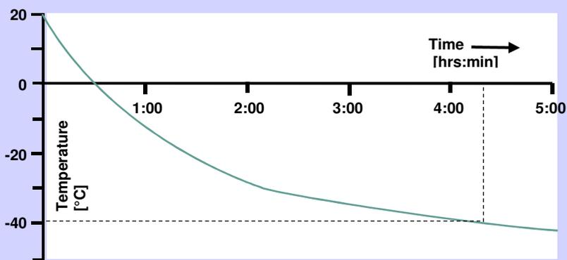
Temperature stability (methanol used as bath liquid)
